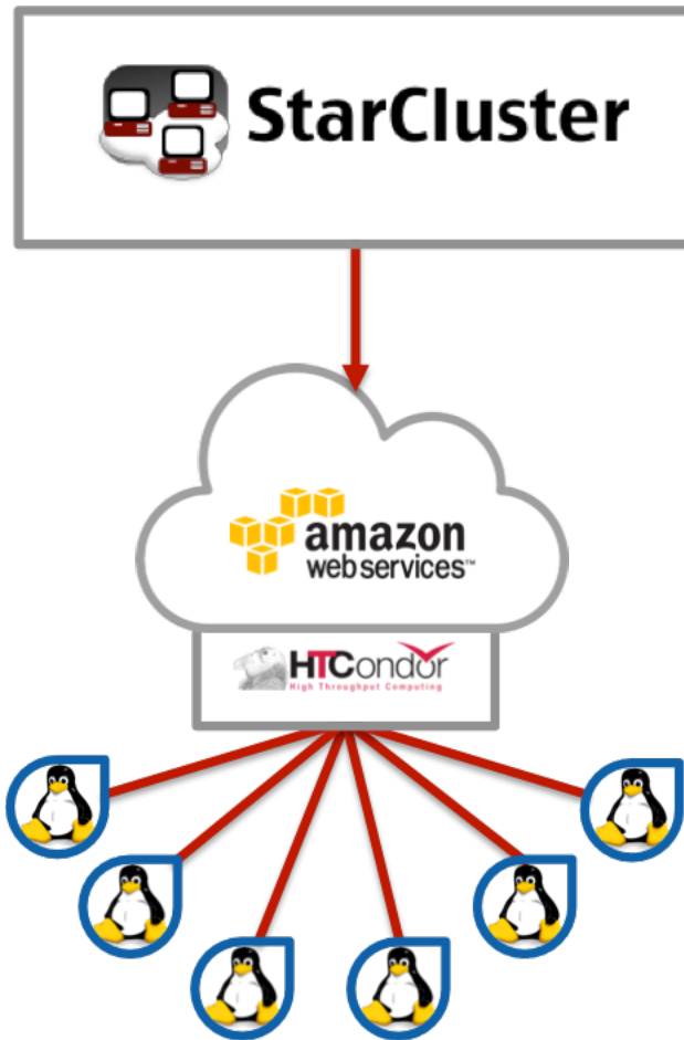
Figure 3-1. StarCluster can provision an HTCondor pool of Linux virtual machines on Amazon Web Services.
